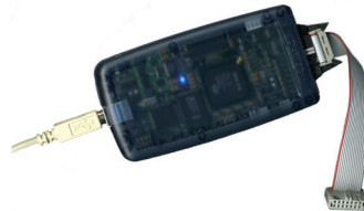
PCI or USB JTAG: These MDS products were specifically designed for Nexperia developers and offers unmatched code download speed.
